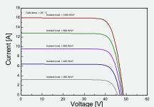
I-V CURVES OF PV MODULE(615W)
